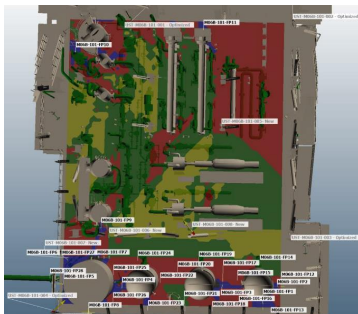
Figure 3 – 2D illustration of flame detectors coverage for detection (blue zones) and emergency actions (red, green and yellow zones) on a fire zone.
